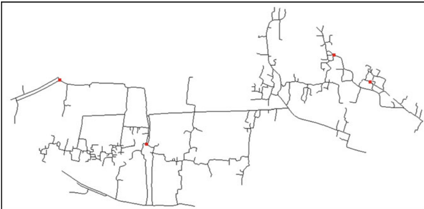
Fig. 11 Position of air valves highlighted in red square bullets
