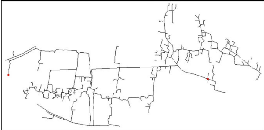
Fig. 12 Position of scour valves highlighted in red square bullets
