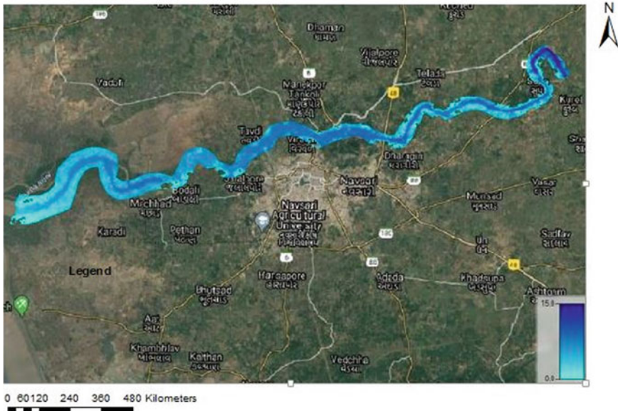
Fig. 7 Simulated flood depth for the 2004 years flood event
