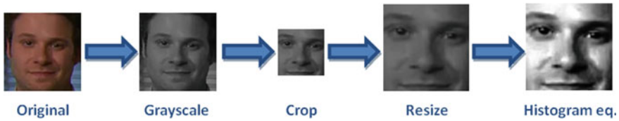
Fig. 3 Preprocessing of the test image
