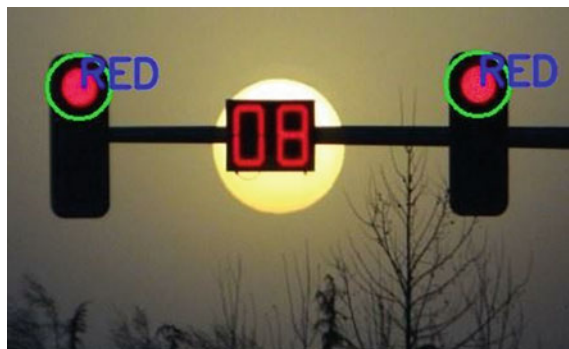
Fig. 7 Snapshot of the detection of red signal color
