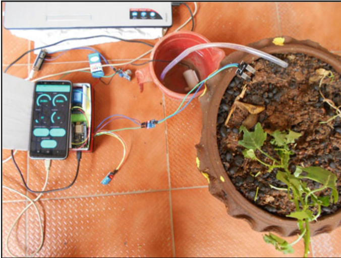
Fig. 10 Hardware implementation (Motor is OFF at High Moisture)
