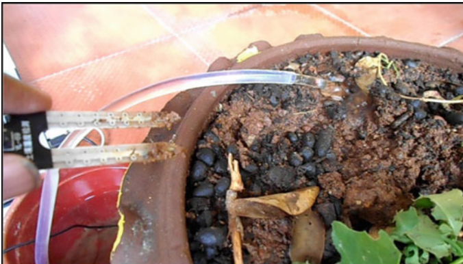
Fig. 11 Hardware Implementation (Motor is ON at Low Moisture)
