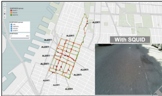
Fig. 4 Result on mobile screen after the device is inbuilt in vehicle and we were able to get consistent image position and accelerometer to differentiate one street from the next in terms of overall quality
