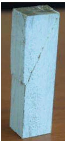
Fig. 13 Failure pattern of Acacia wood test
