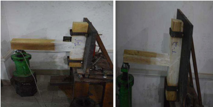
Fig. 9 T-joints subjected to bending in loading frame
