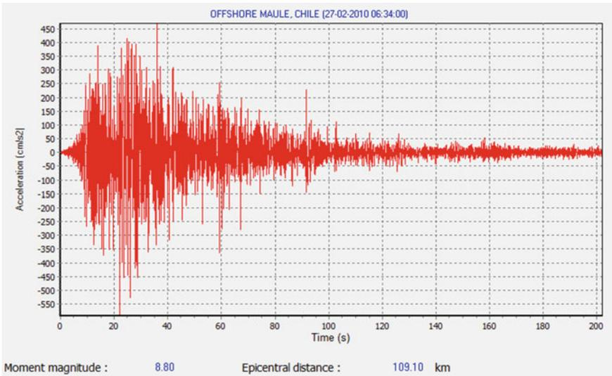
**Fig. 4** Acceleration time history used for the analysis
