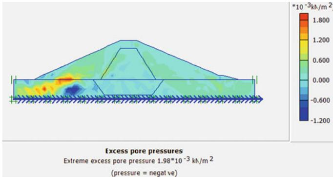
Fig. 13 Excess pore water pressure
