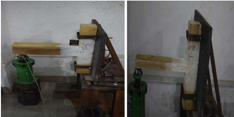
Fig. 9 T-joints subjected to bending in loading frame
