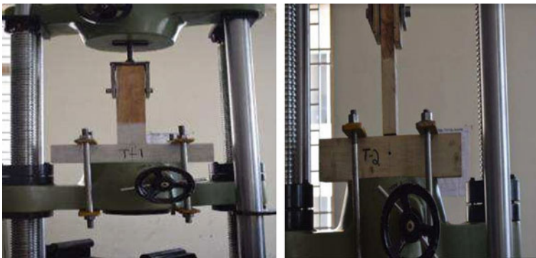
Fig. 10 T-joints subjected to tension test in universal testing machine
