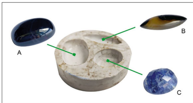
Fig. 2 Silicone rubber mold created with gemstones with different cuts: A cabochon cushion antique cut; B cabochon marquise cut; and C mixed cut
