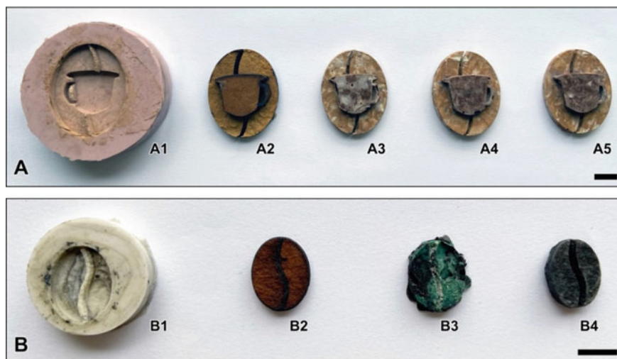
Fig. 6 Manufactured pieces for jewelry application. A Pendant piece production: (A1) silicone mold; (A2) original designed piece in laser-engraved MDF; (A3) first and (A4) second pieces produced with the presence of discontinuities and air bubbles; (A5) third piece without apparent defects. B Ring piece production: (B1) silicone mold; (B2) original designed piece in laser-engraved MDF; (B3) first piece produced with the presence of discontinuities and air bubbles; (B4) second piece without apparent external defects. Scale bars are 10 mm
