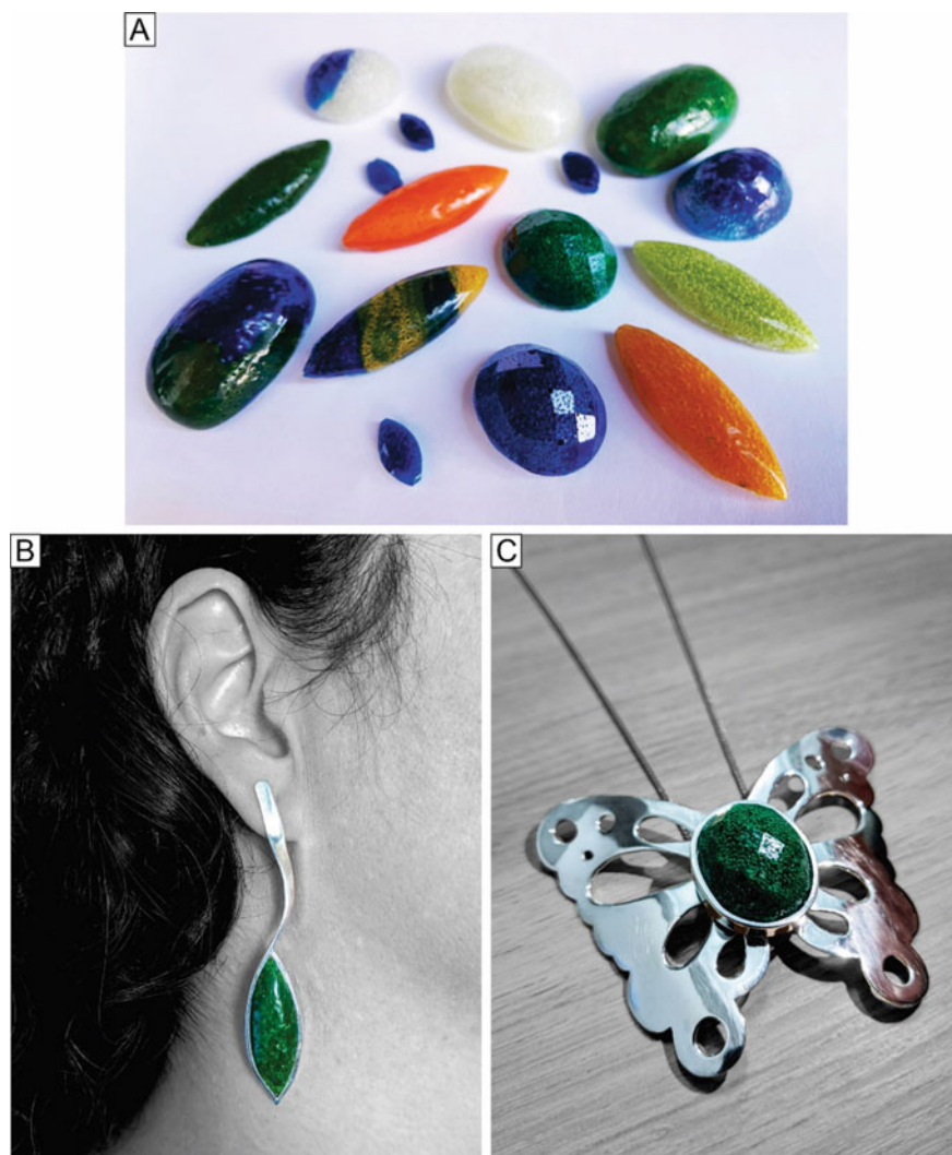
Fig. 4 Recycled EPS packaging for contemporary jewelry: A examples of obtained plastic gemstone pieces with different material colors; B application of a cabochon marquise cut piece with recycled silver into earrings; C application of a mixed cut piece into a pendant with recycled silver
