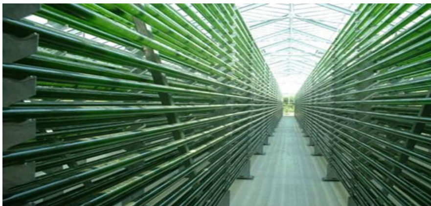
Fig. 10.11 Schematic photobioreactor design that follows a horizontal tube. (Source: Abdel-Raouf N., Al-Homaidan, A. A., and Ibraheem, I. B. (2012). Microalgae and wastewater treatment. Saudi J. Biol. Sci. 19, 257–275. doi: https://doi.org/10.1016/j.sjbs.2012.04.005 . Open access Reprinted with Licence no. 4880801372566 dated 2nd Aug 2020 RightsLink)
