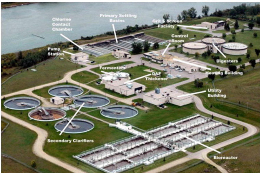
Fig. 10.1 Hybrid technology: Microalgae and wastewater treatment. (Source: Abdel-Raouf, N., Al-Homaidan, A. A., and Ibraheem, I. B. (2012). Microalgae and wastewater treatment. Saudi J. Biol. Sci. 19, 257–275. doi: https://doi.org/10.1016/j.sjbs.2012.04.005 . Open access: Reprinted with Licence no. 4880801372566 dated 2nd Aug 2020 RightsLink)
