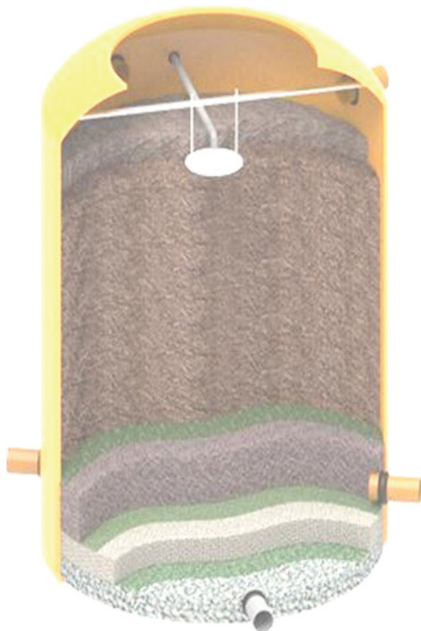
Fig. 18.3 Transversal view Lumbrifilter (NOBATEK/ INEF4 n.d.-b)
