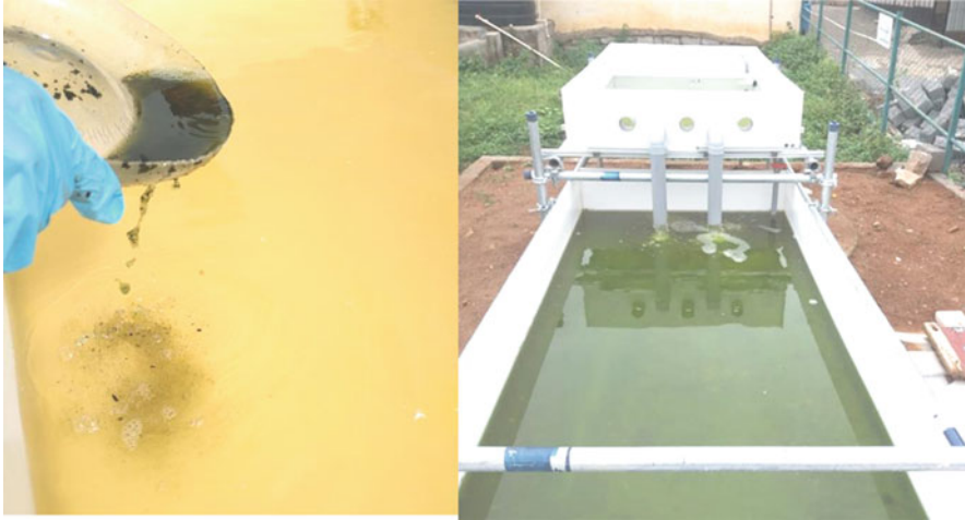
Fig. 18.5 BioSolar Purification, inoculation of algae on Day 0 and Day 10 after inoculation of algae
