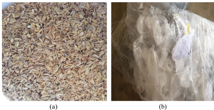
Fig. 1 Material used for manufacturing of NFCs a RH; b LDPE
