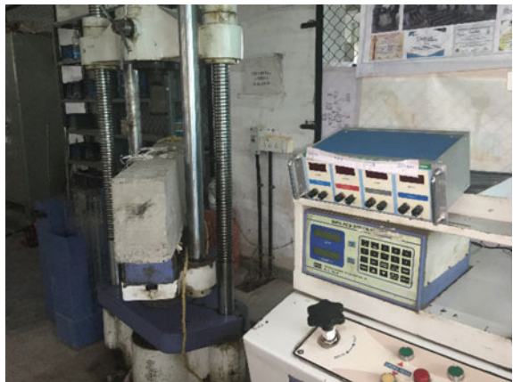
Fig. 9 Two-point load set-up for BRC lintel
