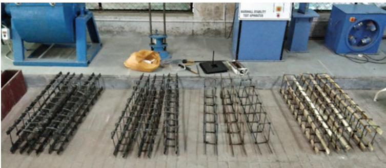
Fig. 2 Treated bamboo cages ready for casting
