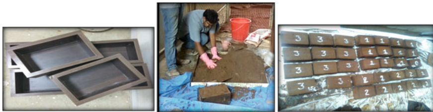
Fig. 5 Molding and casting of adobe blocks
