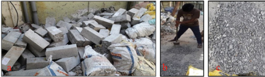
Fig. 3 RCA preparation: a laboratory tested concrete beams, b crushing concrete beam and c crushed concrete beam
