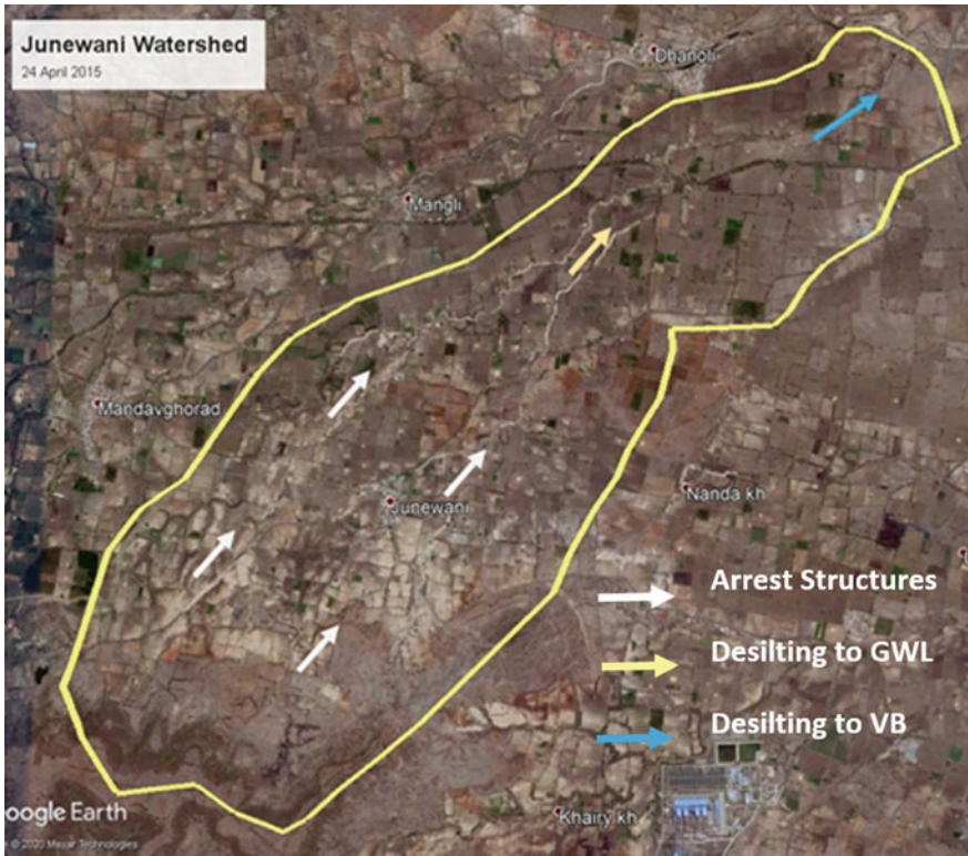
Fig. 8 Overall groundwater dynamics in the watershed and locations of recharge mechanisms to be adopted
