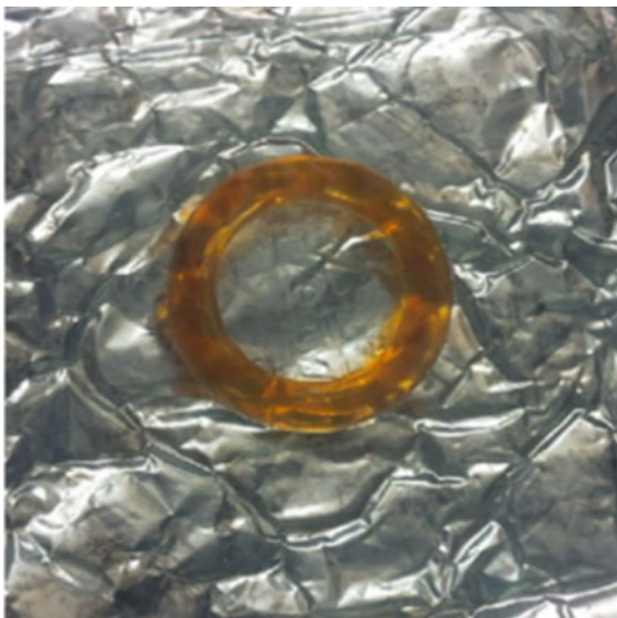
Fig. 5.4 Chitin ring (40 mm diameter) coagulated in antisolvent (water)
