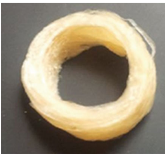
Fig. 5.5 Chitin ring (40 mm diameter) after freeze-drying
