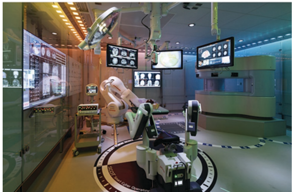
Fig. 53.1 High-performance smart treatment room prototype (hyper SCOT). With the intraoperative MRI as the core, all medical devices are connected by a network, and information is displayed on the navigation in time synchronization. It is also equipped with a robotized microscope, a robotized operating table, and a robot that supports the operator’s hands. A clinical version was installed to start operation at Tokyo Women’s Medical University in 2019
