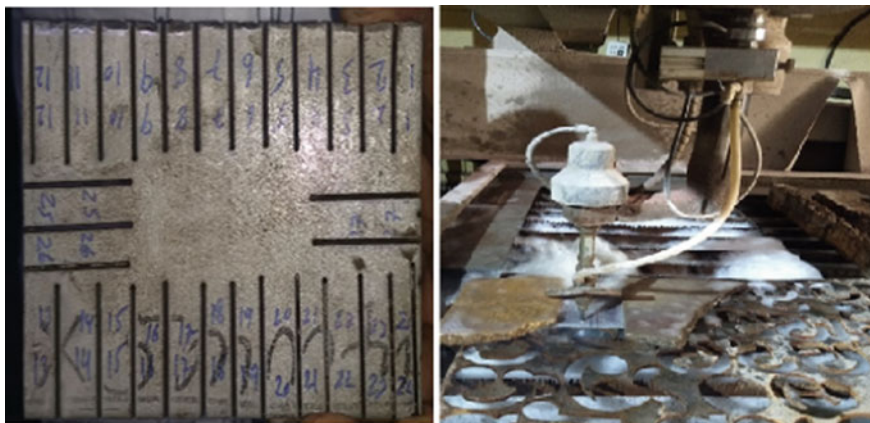
Fig. 2 Nimonic C-263 workpiece and abrasive water jet machine
