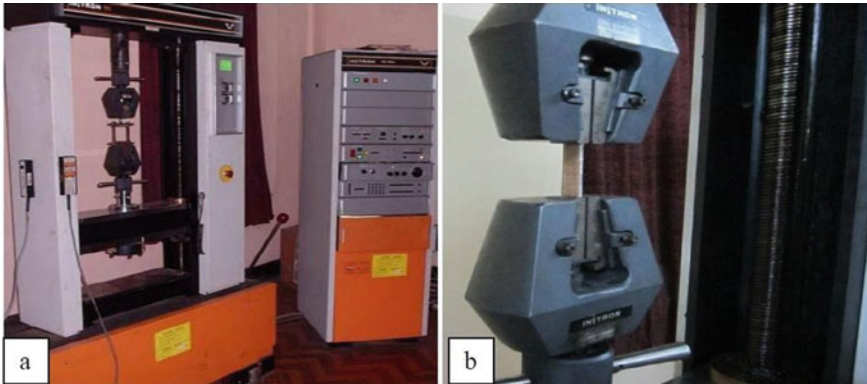
Fig. 5 (a) Experimental setup and (b) loading arrangement of specimen for tensile strength test
