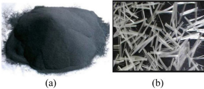
Fig. 1 a Fine greenish silicon carbide powder and b Chopped E-glass fibre
