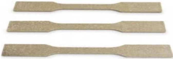
Fig. 7 Tensile test specimen of rice husk and nanoclay-reinforced epoxy composite
