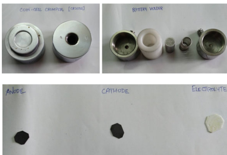
Fig. 6 Illustration of the setup—crimper; used to fix the cells together, battery holder, the prepared anode, cathode and solid biopolymer electrolyte
