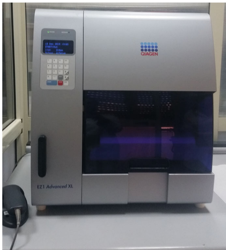
Fig. 2 Example of automated robotic workstation (Author's Property)
