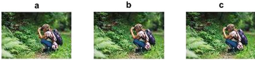
Fig. 9 a Original image (JPEG2000). b Received image through 2-branch MRC with 12 dB transmitted power. c Received image through 3-branch MRC with 12 dB transmitted power
