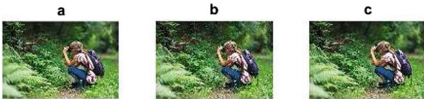
Fig. 8 a Original image (JPEG2000). b Received image through 2-branch MRC with 5 dB transmitted power. c Received image through 3-branch MRC with 5 dB transmitted power
