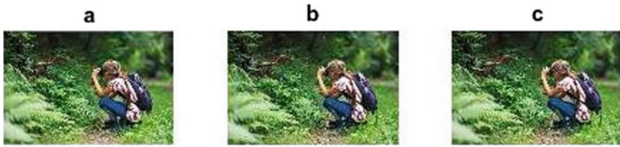
Fig. 5 a Original image (JPEG2000). b Received image through 2-branch SC with 12 dB transmitted power. c Received image through 3-branch SC with 12 dB transmitted power
