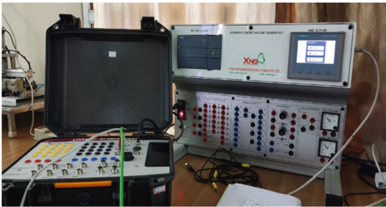
Fig. 3 PLC connected to data logger
