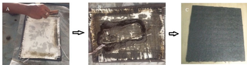
Fig. 1 a Laminas of E-glass fiber, b applied Haritaki Epoxy mixing resin, c finished fabrication of laminated composites
