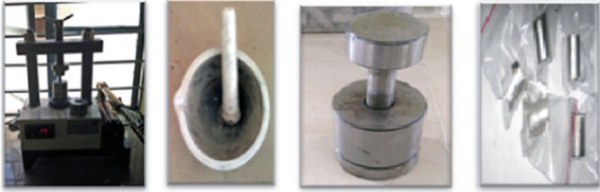
Fig. 2 Compaction press, crucible, die and ejected specimen
