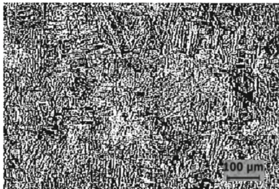
Fig. 1 Optical microstructure of substrate material at 100X magnification
