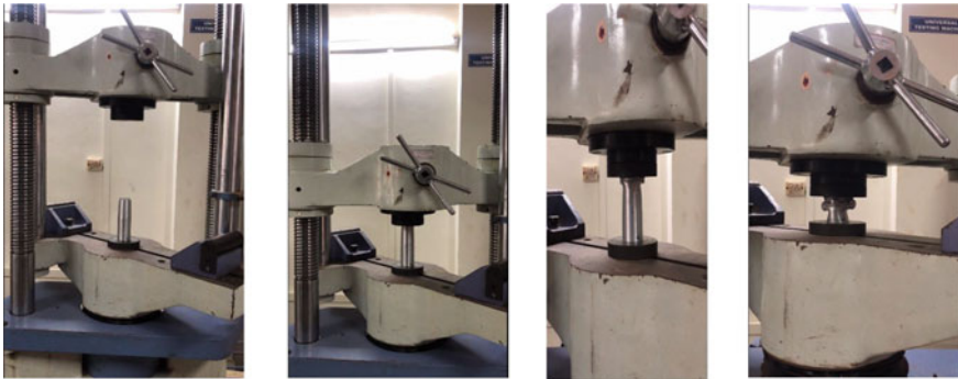
Fig. 5 Sequence of deformation of UT tubes obtained through experiments
