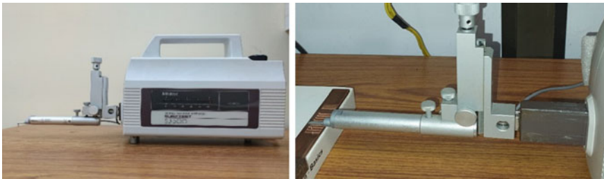
Fig. 2 Surface roughness tester and measurement arrangement
