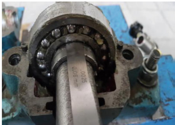
Fig. 3 Sleeve and inner race clearance of 0.04 mm
