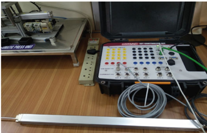
Fig. 4 Balluff sensor connected to Data Logger
