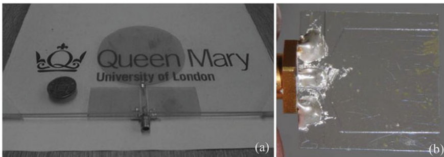
Fig. 2 a A ultra-wideband transparent disc antenna. b A compact size ultra-wideband transparent antenna
