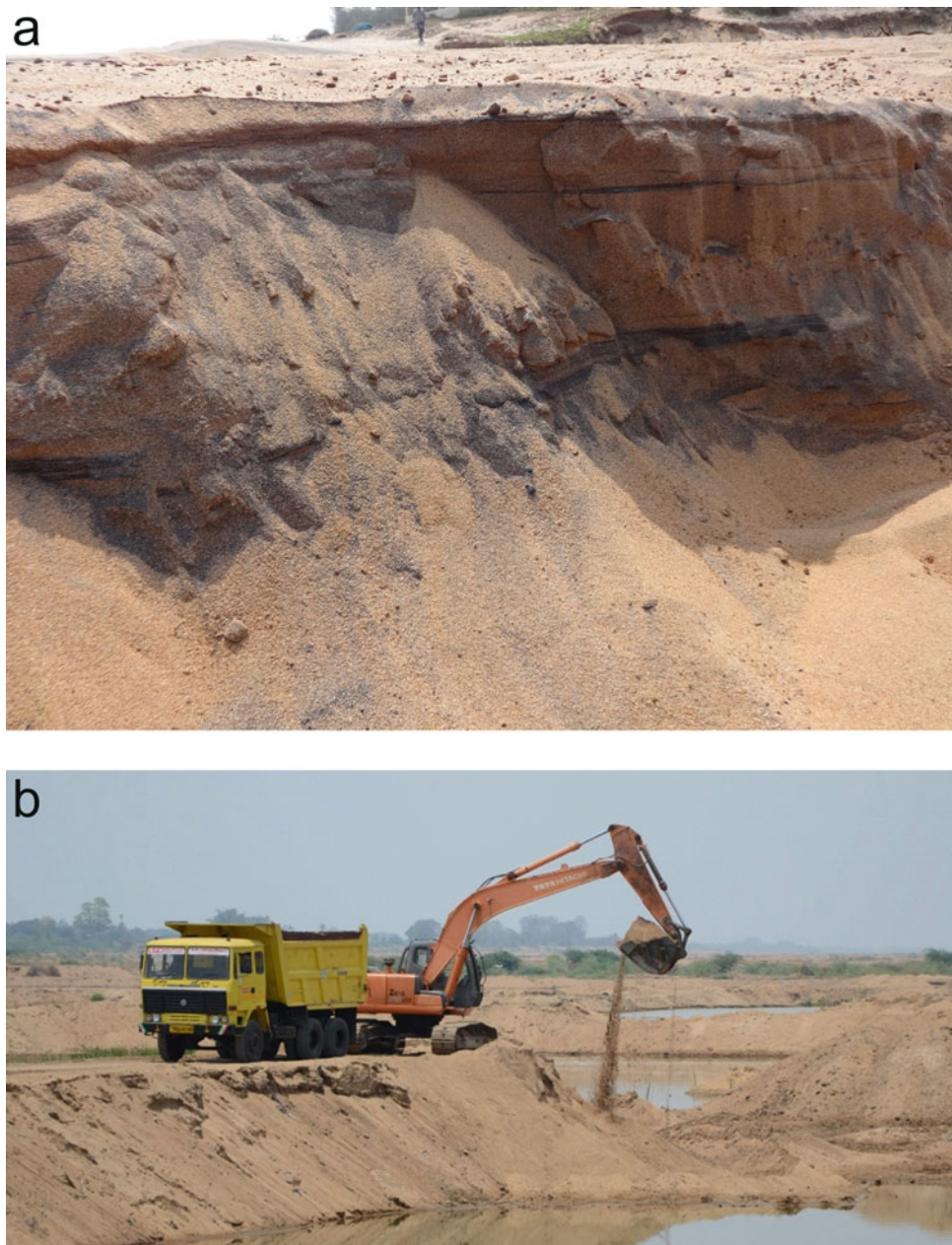
Fig. 6 Extensive beach sand deposits: a General view of beach sand deposit with prominent layers of heavy minerals (black); b Mining of a vast stretch of beach sand deposit by deploying JCB (Credit Deepak Rathod)
