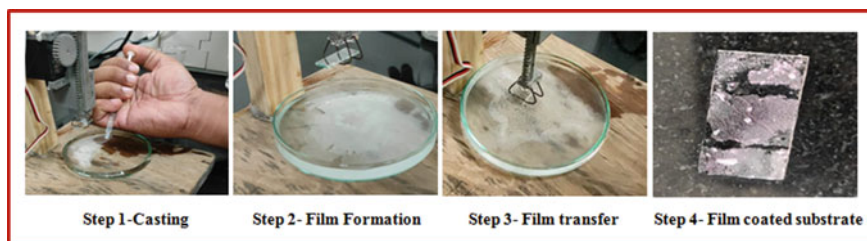
Fig. 6 Photographic images captured during film formation and transfer process
