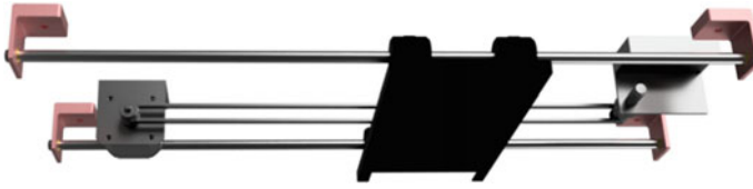
Fig. 3 Isometric view of slider mechanism
