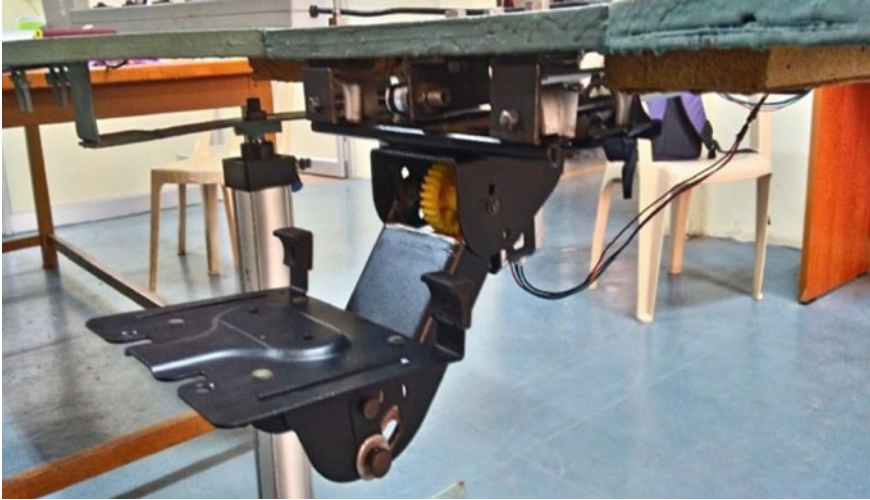
Fig. 9 Fabrication of an automated tray mechanism
