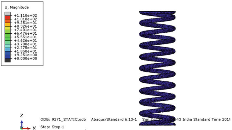
Fig. 6 Deflection of the spring model 1
