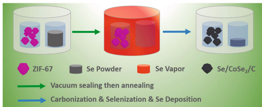
Fig. 2.16 An illustration of the single-step carbonisation and selenisation treatment of ZIF-67 with the Se powder in a vacuum-sealed glass vessel, leading to the formation of MOF-derived \text{Se/CoSe}_2/\text{C} composite. Reproduced with permission [90]. © 2019 Elsevier
