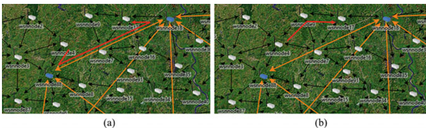
Fig. 32.6 Comparison of the links between adjacent nodes in adjacent clusters: a Use the classic clustering routing protocol for WSN; b Use CTM routing protocol for WSN
