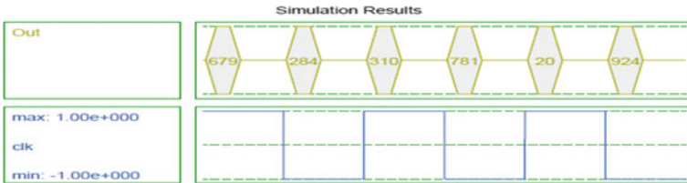
Fig. 5 Simulation outcome of proposed 8-bit TRNG from QCA Designer
