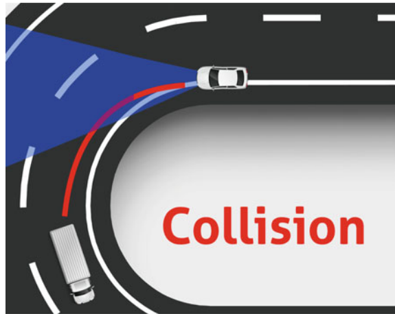
Fig. 41.2 Overtaking a heavy-duty vehicle without adaptive vehicle safety system
