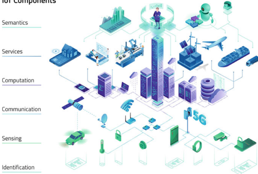
Fig. 19.1 IoT architectural components
