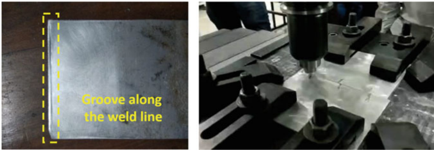
Fig. 1 The groove along the weld line of 7075 aluminium alloy (left) and the tool set up of for FSW of 7075 aluminium alloy (right)
