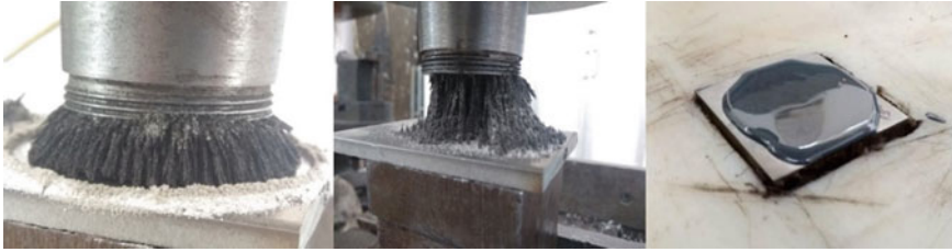
Fig. 3 FMAB and media on the workpiece without the magnetic field
