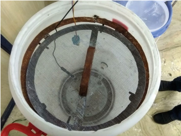
Fig. 5 Screening system of steel wire mesh is used for primary stage in prototype model
