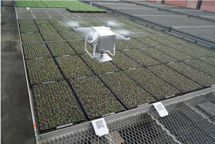
Fig. 5.7 Photograph illustrating a drone connected to a compact GaN semiconductor microwave generator with an antenna used to continuously apply a microwave irradiation pattern to the plants [8]
