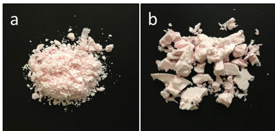
Fig. 14.23 Freeze-dried Pickering double emulsions with encapsulated carmine using solid shea nut oil (melting point 33 °C): (a) non-heat-treated freeze-dried double emulsion and (b) heat-treated freeze-dried double emulsion on the right, reprinted with permission from Marefati et al. (2015)
