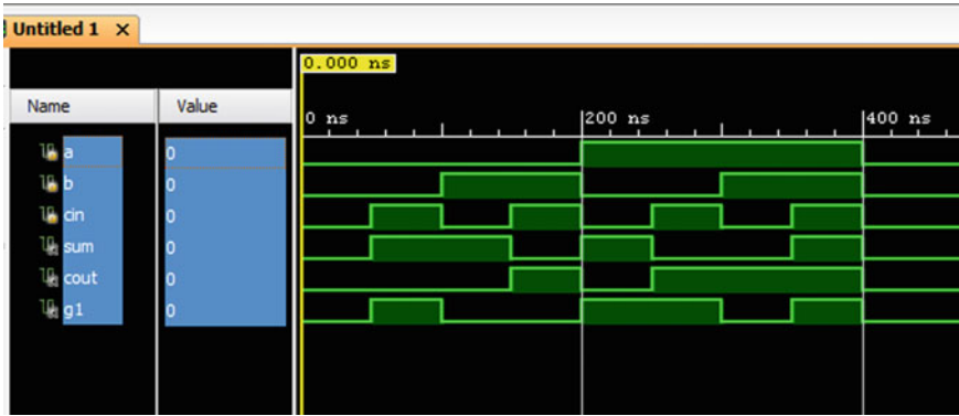
Fig. 9 Simulation waveform of full-adder
