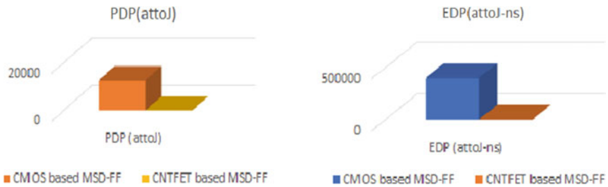
Fig. 7 PDP and EDP comparison between CMOS- and CNTFET-based MSD-FF
