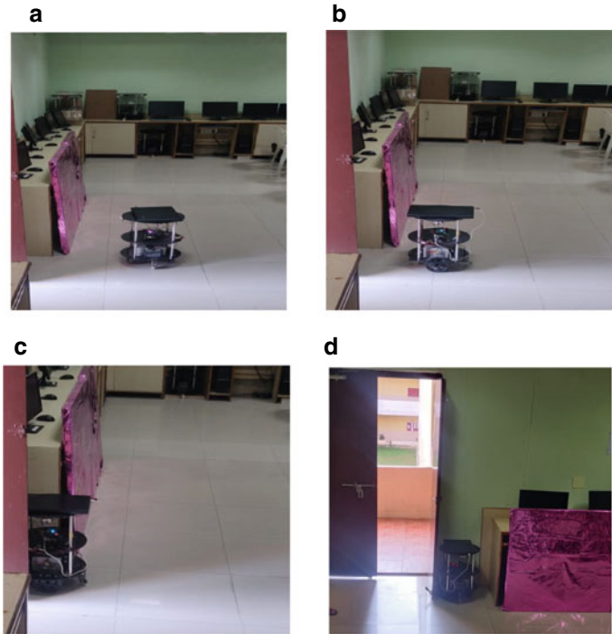
Fig. 3 a-d: Snap shots of FPGA-based mobile robot parallel parking
