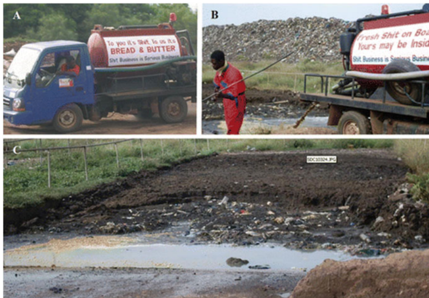
Fig. 7.1 Human fecal sludge for agriculture: fecal sludge being delivered (a) and discharged (b) to a dewatering (drying) bed (c) in Accra, Ghana. The signs on either side of the truck indicate the value of fecal sludge as a resource (Hamilton et al. 2014)
