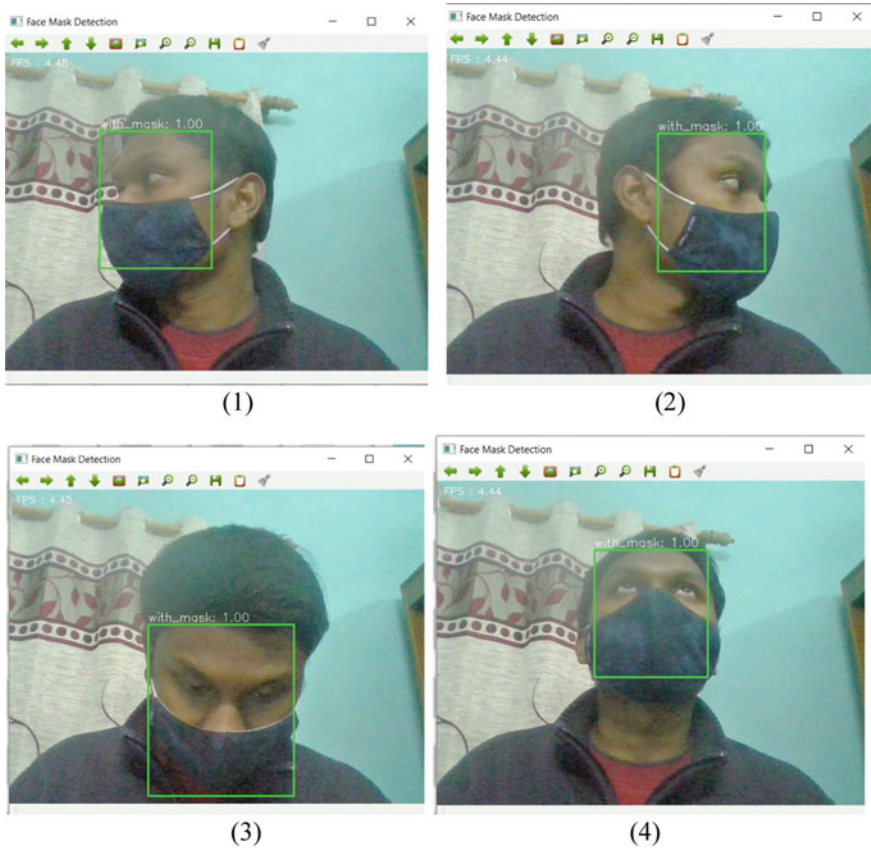
Fig. 14 Side face view mask detection (1), (2), and vertical head movement (3), (4) tracking using MTCNN face detector
