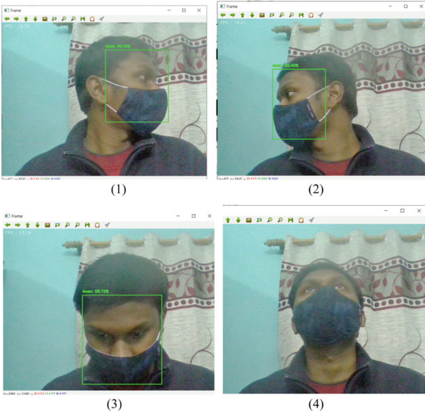
Fig. 13 Side face view mask detection (1), (2), and vertical head movement (3), (4) tracking using Caffe model face detector
