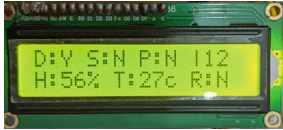
Fig. 9 Output displayed on LCD (sensors values)
