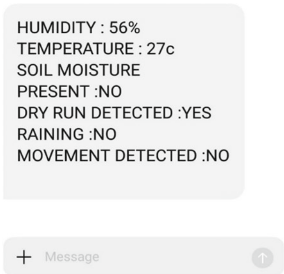
Fig. 10 Output via mobile SMS (sensor values)
