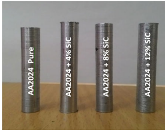
Fig. 8 Fabricated wear pins
