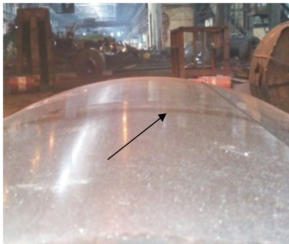
Fig. 7 Photograph of outer layer of a CR coil having ridge defect
