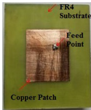
Fig. 8. Fabricated conventional MSTPA
