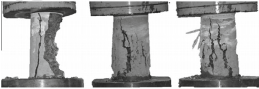
Fig. 11 Effect of the rubber sand on concrete cracking failure test in concrete based pavements, a zero rubber sand, b 20% rubber sand, c 40% rubber sand. Reprint with the permission of Elsevier 2014 (Mohamaddi et al. 2014)
