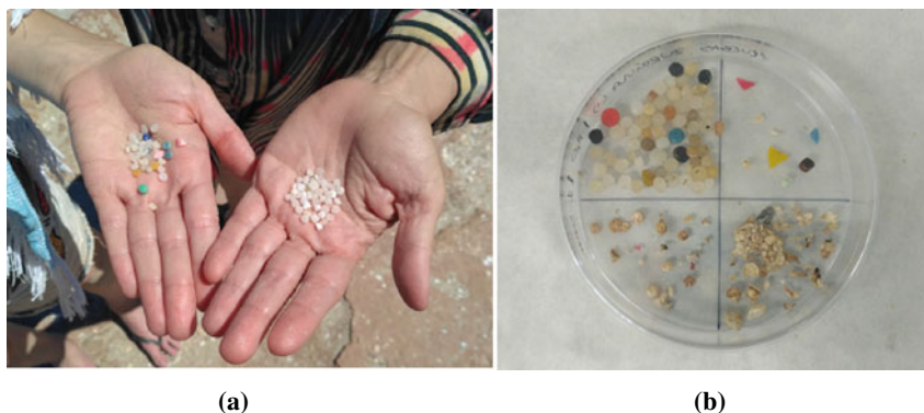
Fig. 6 Photographs of a primary MPs, constituted by industrial pellets recovered from a beach, and b primary and secondary MPs
