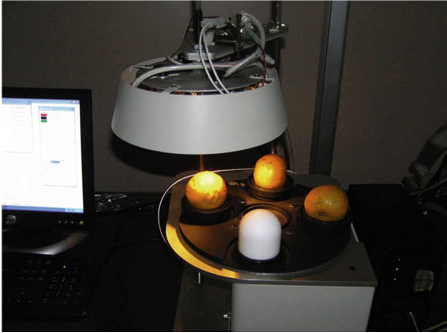
Fig. 10.9 The NIR spectra collection of Thai oranges from spectrometer (model: PureSpec, Saika Technological Institute Foundation, Japan)
