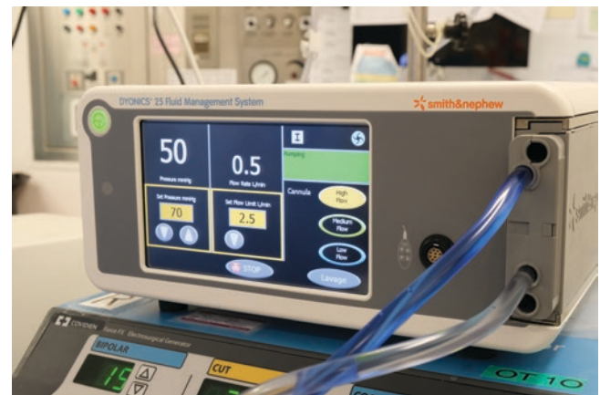
Fig. 3.4 Automated peristaltic fluid pump systems with pressure and flow regulation
