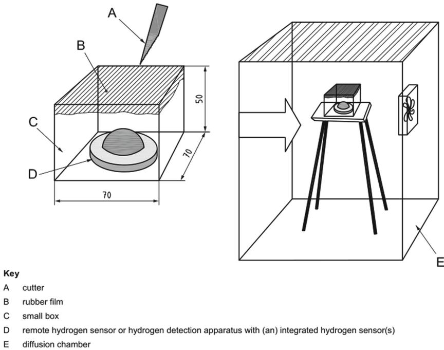
**Fig. 1.** Small box used for response time
