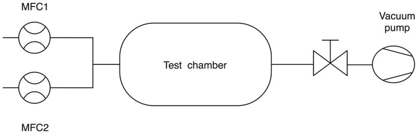
**Fig. 2.** Gas control schematic diagram
