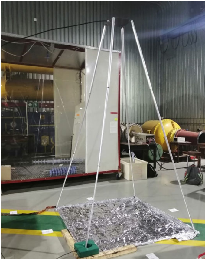
Fig. 3 Lightning safety structure for individual occupation (Constructed and tested by Mr. Musa T. Mukansi and Mr. Mathew L. Woodhead, School of Electrical and Information Engineering, University of Witwatersrand, South Africa)
