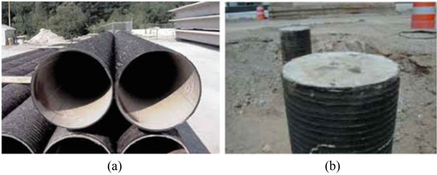
Fig. 2 FRP composite pile a hollow FRP pipe and b concrete-filled FRP pile [1]
