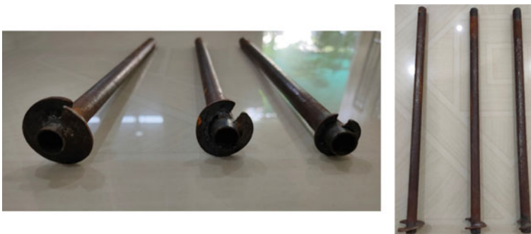
Fig. 4 Model helical pile used in experimental investigation
