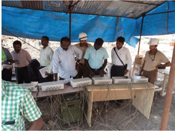
Fig. 3 Instrumented vertical load test—data collection in progress
