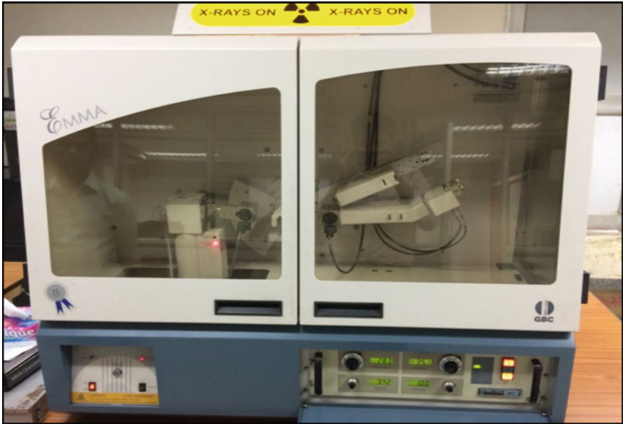
Fig. 5 Mineralogy study with XRD
