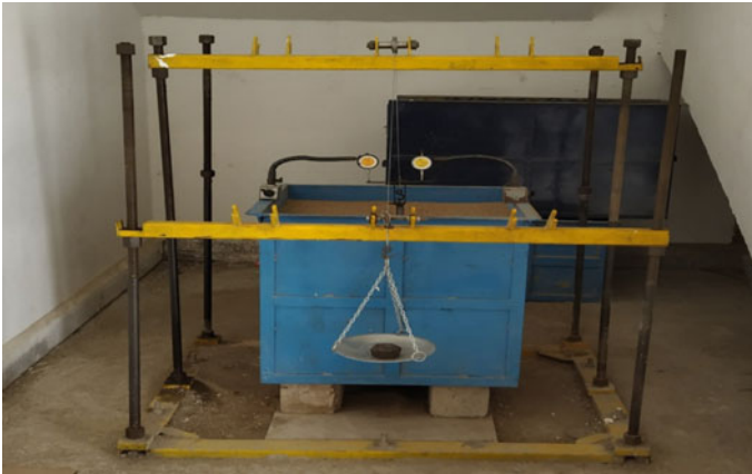
Fig. 3 Test setup for uplift loading on helical pile
