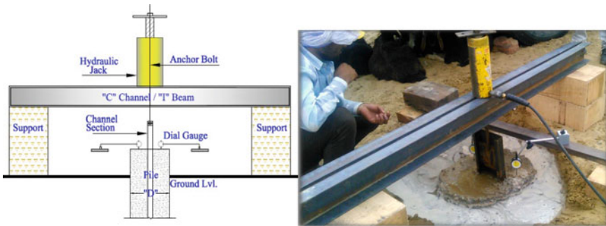
Fig. 8 Test arrangement for pile pullout test. Sketch on left is a schematic of the test setup. Photo on right shows test in progress
