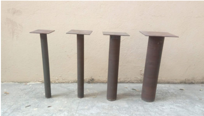
Fig. 1 Steel pipe piles
