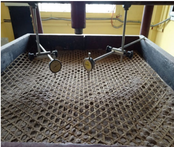
Fig. 8 Hexagonal aperture bamboo mat at required depth
