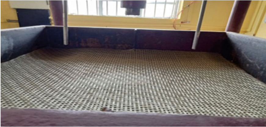
Fig. 5 Square aperture bamboo grid at required depth
