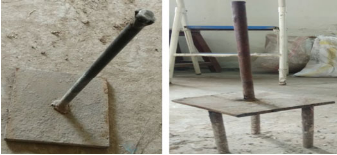
Fig. 3 Fabricated micropile system includes a footing plate with micropile (left) and footing plate with three micropiles (right)
