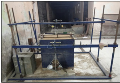
Experimental Setup used for uplift Load-ing
