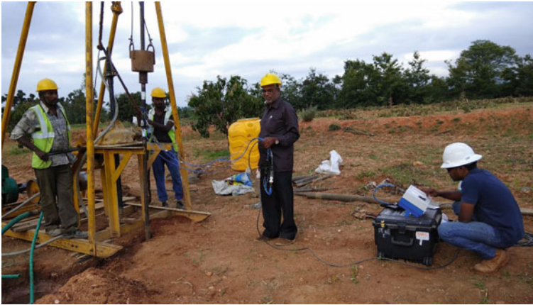
Fig. 4 SPT Energy measurements at Site-A
