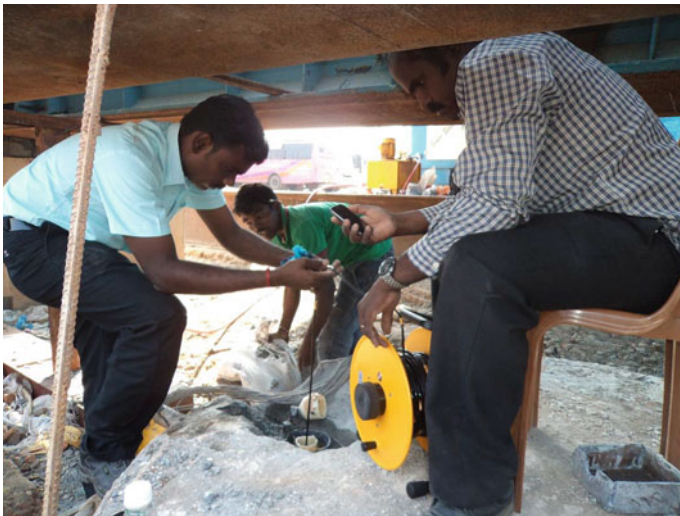
Fig. 7 Inclinometer reading being taken during lateral load test
