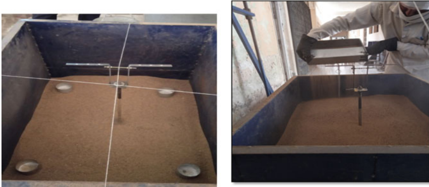
Fig. 3 Preparation of sand bed using rainfall techniques
