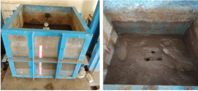
Fig. 6 Set-up for the heave test with dial gauge arrangement (left), and heave action of soil after four days (right)
