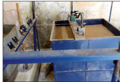
Experimental Setup used for Lateral Loading
