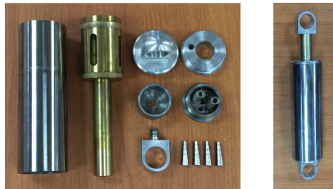
Fig. 5. SMA damper prototype and its decomposed components.
