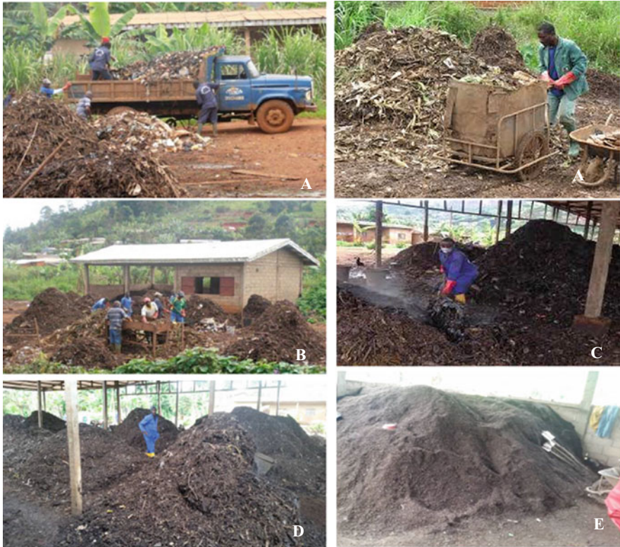
Fig. 9.7 Composting process. (a) Waste supply, (b) sorting of waste and piling up, (c) turning heaps, (d) pile of compost under shelter, (e) compost dry sieved. Source: (a)–(c) (Ngnikam 2013); (d) and (e) (author's picture)
