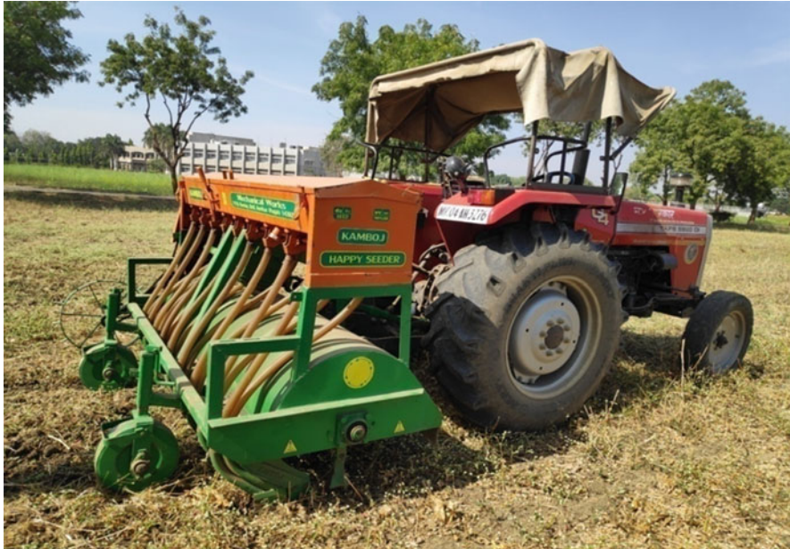
Fig. 8.7 Turbo Happy Seeder for the sowing of crops in residue retained fields under conservation agriculture
