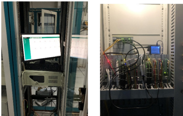
Fig. 10. On-site deployment diagram of servers and gateways
