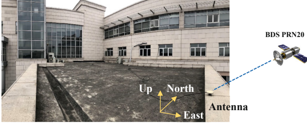
Fig. 3. SJTU microelectronics building terrace environment photo, a multipath signal from Beidou PRN20 satellite (elevation 16.8°, azimuth 61.1°) is detected.
