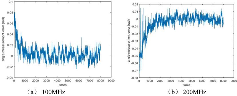
Fig. 5. The angle measurement error of different frequency (a) 100 MHz; (b) 200 MHz
