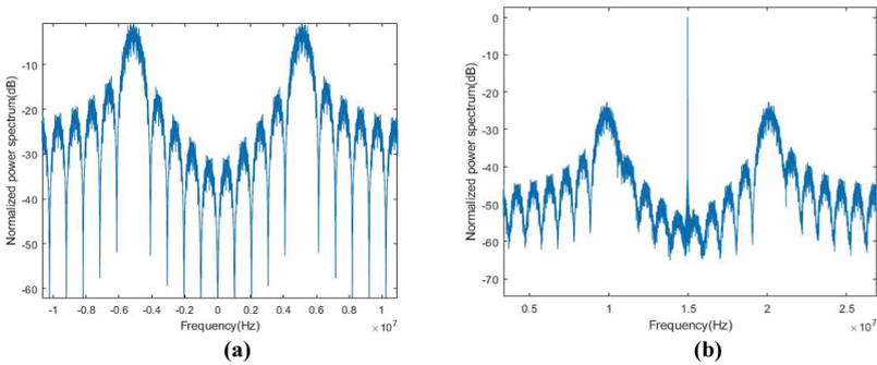
**Fig. 3.** Normalized power spectrum of transmitted signal. (a) Normalized power spectrum of base-band BOC (5, 1) signal; (b) Normalized power spectrum of intermediate frequency signal
