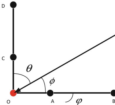
**Fig. 4.** Diagram of orthogonal baseline phase interferometer
