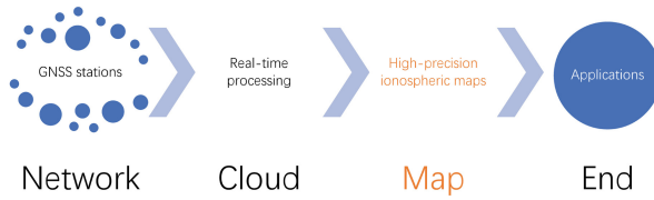
Fig. 1. Architecture of ionospheric real-time monitoring system
