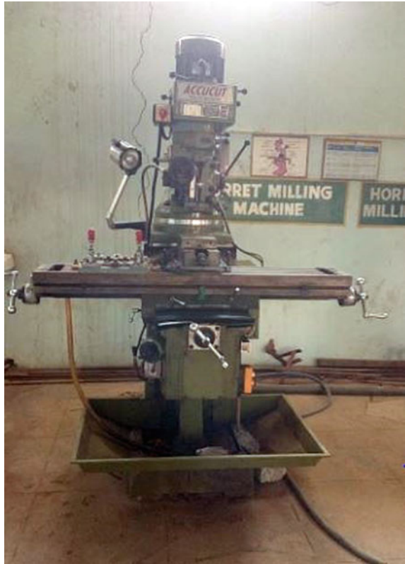
Fig. 2 Accucut milling machine used during FSW process
