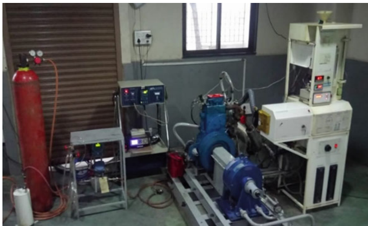
Fig. 1 Experimental set-up used with hydrogen supply and safety system
